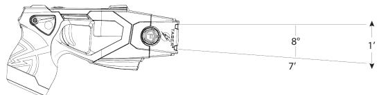
The bottom probe impacts at an 8-degree angle from the top probe. This results in a spread of approximately 1 foot (0.3 m) for every 7 feet (2.1 m) of distance from the energy weapon. Greater probe spread increases effectiveness.
