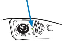
An orange LED indicates a “low” battery. In some conditions, especially low temperature (–4 °F/–20 °C) the LED may display orange even if the battery has sufficient charge left.
